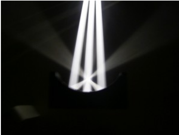
Image : Beam path in a concave mirror. By Johannes S., License: CC BY-SA 3.0
