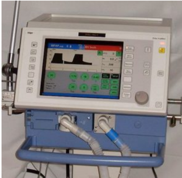
Image: "Respirator "Evita4" in an ICU." by Blogotron – Own work. License: CC0
